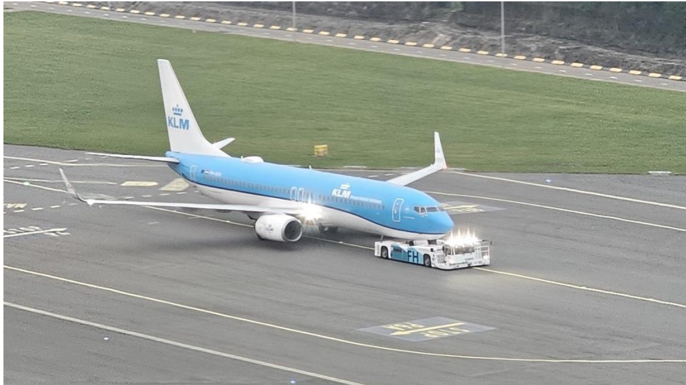
Fig. 3. A KLM B737-8MAX with the TaxiBot, at the end of its taxiing phase to RWY 36L (Polderbaan RWY). Photo taken by Benjamin van der Sanden.
