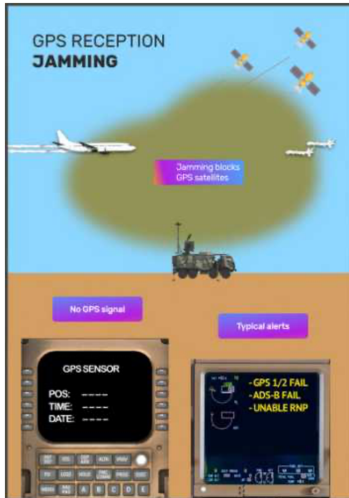
What is Jamming? How does it work and what display can be expected in the flight deck. (OPS Group, 2024a)
